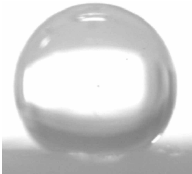
Figure 5. Photographs showing a water droplet on the surface of silica aerogel-fiber composites dried at ambient pressure (the contact angle = 135^\circ ).
